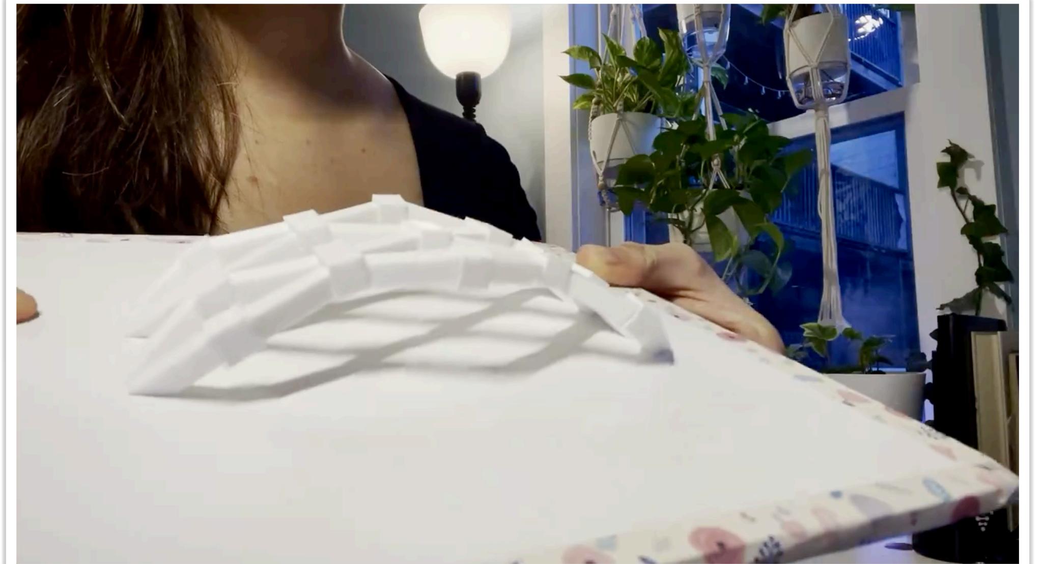
a push puppet-inspired deployable structure by Lin and Tachi
