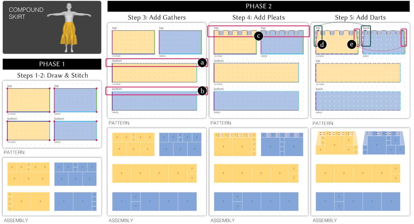
Figure 10: To draw a two-layer compound skirt in REFASHION Studio, the user starts by drawing and stitching panels to form the base pattern as shown in Phase 1 (Steps 1-2). In Phase 2, they manipulate its shape by adding features. First (Step 3), they gather edges (a) and (b) to add volume to the second layer of the skirt. Next (Step 4), they convert every other unit along its waistline (c) into right-folding pleats to cinch the waist. Finally (Step 5), they add darts (d) and (e), which align across the side seams, to refine the waist-to-hip shaping. For each step, we display both the resulting pattern (top) and its corresponding assembly (bottom). The simulation is in the upper left.
